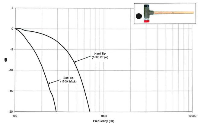
PCB<sup>®</sup> impulse hammers are available in sizes ranging from the mini-impulse hammer to the 12 lb sledgehammer. All sensors in this system are classified as ICP<sup>®</sup> (Integrated Circuit Piezoelectric), low impedance, voltage-mode sensors. Microelectronic, built-in amplifiers standardize sensitivities within a few percent of nominal value, which is adequate for most dynamic applications.
