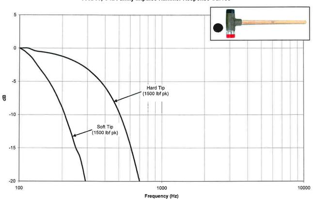
PCB<sup>®</sup> impulse hammers are available in sizes ranging from the mini-impulse hammer to the 12 lb sledgehammer. All sensors in this system are classified as ICP<sup>®</sup> (Integrated Circuit Piezoelectric), low impedance, voltage-mode sensors. Microelectronic, built-in amplifiers standardize sensitivities within a few percent of nominal value, which is adequate for most dynamic applications.
