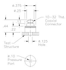
Models 103A02 and 103A12: ICP® Sound Pressure Sensors
