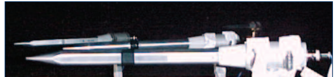
FIGURE 9: Wrap of Tape around Probe Sensing Face
