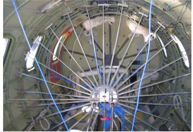
Fig 1. Circular microphone array, PCB Microphone model T130D21
