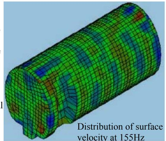
Distribution of surface velocity at 155Hz
