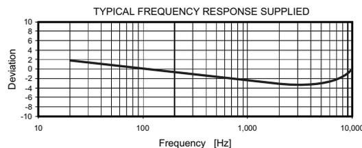
The Endevco® model 2222D is the world's most popular miniature piezoelectric accelerometer for vibration measurement on mini-structures and small objects. Its light weight (1 gm) minimizes mass loading. The accelerometer is a self generating device that requires no external power source for operation.
