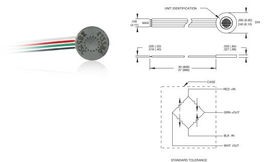
STANDARD TOLERANCE INCHES (MILLIMETERS) .XX = +/- .03 (.X = +/- .8) .XXX = +/- .010 (.XX = +/- .25)
