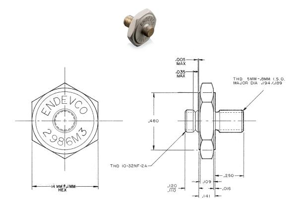
Isolated mounting adapter with 14mm hex for use with accelerometers with a 10-32 thread.
