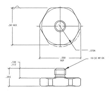
Adhesive mounting base with ½ inch hex for use with accelerometers with a 10-32 thread.
