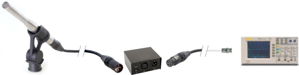
Phantom Powered Microphone System
