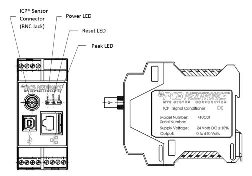
The Power LED is Green, which turns on when the unit is powered. The Reset LED is Green which turns on when both terminals of Reset (Reset + and Reset – are electrically connected to one another). The Peak Hold LED remains Green as long as the unit is powered and not in Reset Mode.
