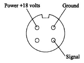
Figure 3: Input Connector Pin Diagram
