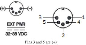
Pins 1, 2 and 4 are (-) Outside shell is earth/chassis ground
