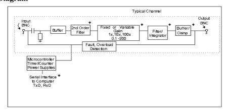
Figure 1 Generic block diagram of model series 482C signal conditioners (\* = option)
