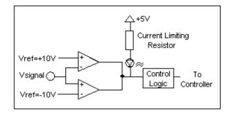
Figure 5 Auto scale/Overload Window Comparator
