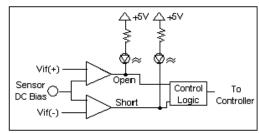
Figure 3 Input Fault Window Comparator with LED Indicator
