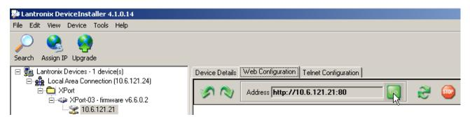
Navigate to the actual device as shown in the left panel above and then click on the 'Web Configuration' tab and clock on the 'Go' button. This will cause the following screen to appear, just select 'OK'. There are no login parameters defined.
