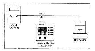
Figure 19. DC Bias Voltage Measurement
