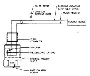
Figure 2. Typical ICP<sup>®</sup> Sensor System
