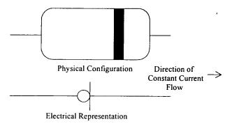
Figure 3. Constant Current Diode
