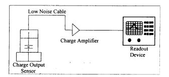
Figure 16. High Impedance System Connection
