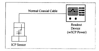
Figure 17. ICP<sup>®</sup> Sensor System Connector
