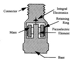
Figure 1. Typical ICP<sup>®</sup> Industrial Shear Mode Accelerometer
