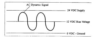
Figure 18. Sensor DC Bias Voltage
