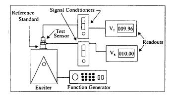
Figure 14. Typical Back-to-Back Calibration System
