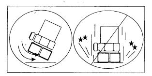
Figure 10. Magnet Mounting
