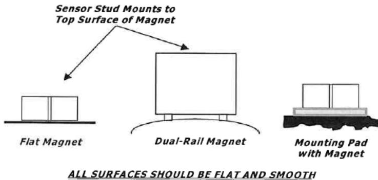
**STEP 1** After choosing the correct magnet type, inspect the unit, verifying that the mounting surfaces are flat and smooth.
