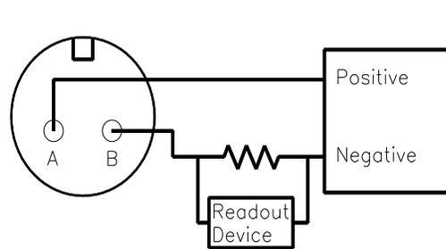
If using a standard DC power supply, install either an ammeter and/or load resistor in line with the output, Pin B or **Blue** Wire.
