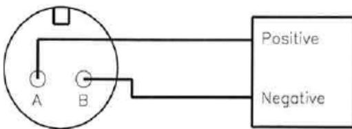
*Figure 2 – wiring: loop powered/DC source*
