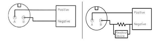
If using a standard DC power supply, install either an ammeter and/or load resistor in line with the output, Pin B or **Blue** Wire.
