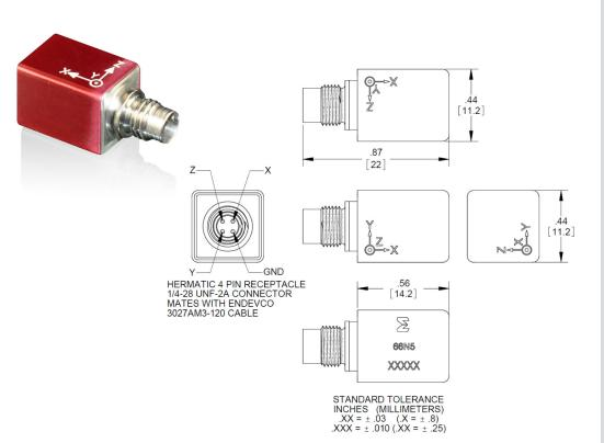
Endevco models 66N5 and 66N6 are miniature triaxial piezoelectric accelerometers with integral hybrid electronics with transducer electronic data sheet (TEDS) capabilities. The accelerometer is packaged in an inner case of welded titanium construction with an outer anodized aluminum case to provide electrical case isolation. One of the key design characteristics is the low unit-to-unit phase deviation at low frequency, ideal for modal analysis of large rigid bodies.
