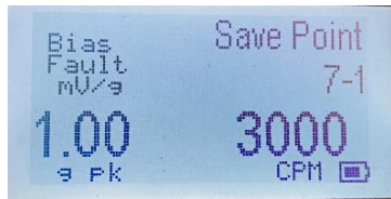
Test Point 4: Known Vibration = 1.00 g pk at 3000 CPM
