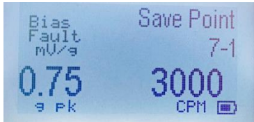
Test Point 3: Known Vibration = 0.75 g pk at 3000 CPM
