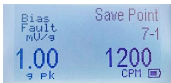
Test Point 2: Known Vibration = 1.00 g pk at 1200 CPM
