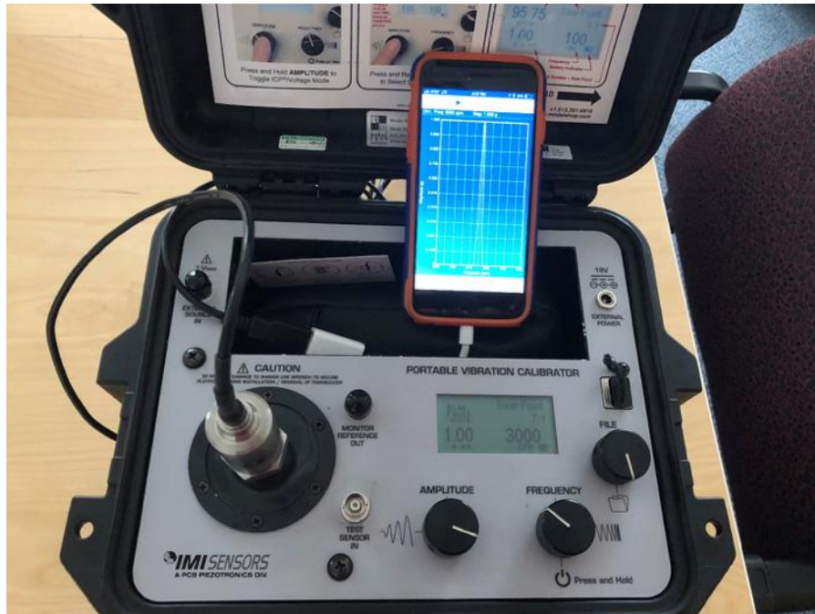
Figure 3: Test Setup – Model 633A01 is mounted onto Model 699B07 Portable Vibration Calibrator; the output of 633A01 is measured using the Signal Scope Pro application by Faber Acoustical
