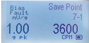
Test Point 5: Known Vibration = 1.00 g pk at 3600 CPM
