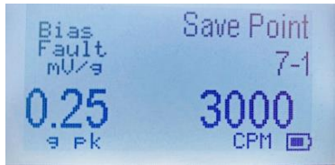
Test Point 1: Known Vibration = 0.25 g pk at 3000 CPM
