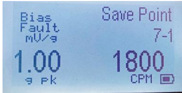
Test Point 3: Known Vibration = 1.00 g pk at 1800 CPM
