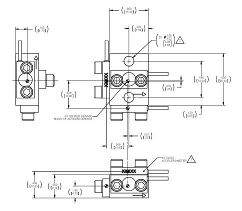
Mounts with provided 6-32 screws, includes 4-40 threaded holes for accelerometer screws.
