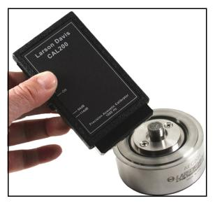
FIGURE 2-4 Installing the CAL200 on AEC201
