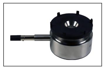
FIGURE 3-6 Type 2 adapter installed on AEC201
