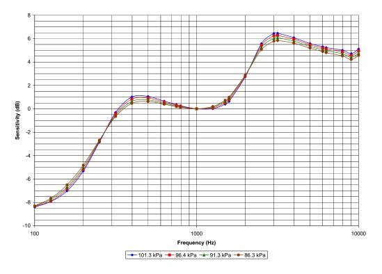
FIGURE A-13 Sensitivity change with Static Pressure Graph
