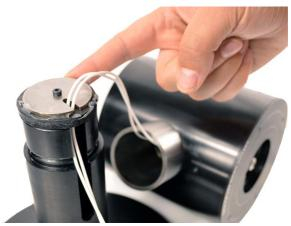
**Step 9** Feed the slack of the cables into the head. Ensure all cables are all the way in before moving on to the next step, if the
