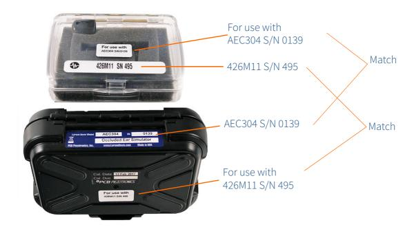
The AEC304 will already be assembled in the head of the AEC206 test fixture. Larson Davis recommends that the entire system be shipped for factory calibration, however, the following procedures describe removing the ear simulator and preamplifier to ship to Larson Davis separately. It is important to reassemble using the steps below exactly in order to maintain acoustic quality, see 2.3.3 "Assembling AEC304" on page 2-7.
