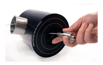
**Step 8** Separate the 426M11 from the AEC304 by unscrewing the two devices. Do not unscrew the ear canal extension.
