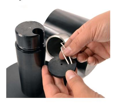
**TAKE NOTE** Align the gasket slit with the center of the cavity in the neck, so the cables run down into the neck.
