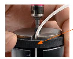
Squeeze the slit in the gasket shut as you tighten the screw.
