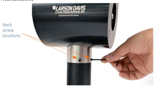
**Step 12** Ensure the AEC304 is completely pushed into the head. Using a torque screwdriver set to 40 oz-in, turn the set screws on the head until push rod is clamped.
