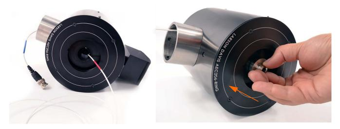
**Step 3** Using the 2.5 mm hex driver, unscrew the washer/gasket screw completely. Pull off assembly, and then separate the washer from the gasket.
