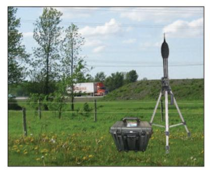
When making outdoor noise measurements, sensitive microphones and noise measuring equipment can be exposed to all types of weather including rain, dew, wind and heat. Protect your equipment and data from the negative effects of exposure to weather by using an Environmental Protection System, EPS. Our EPS products allow a sound level meter to be placed in a protective case and connected to an outdoor microphone system through a watertight orifice using an extension cable.
