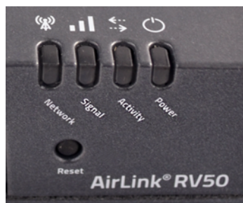
Figure 3-14 Gateway Status Indicators
