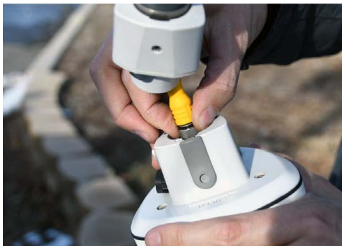
FIGURE 4-11 Feed CBL229-20 Through Weather Arm
