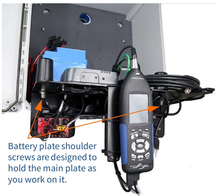
FIGURE 3-5 831C-045 on Shoulder Screws
