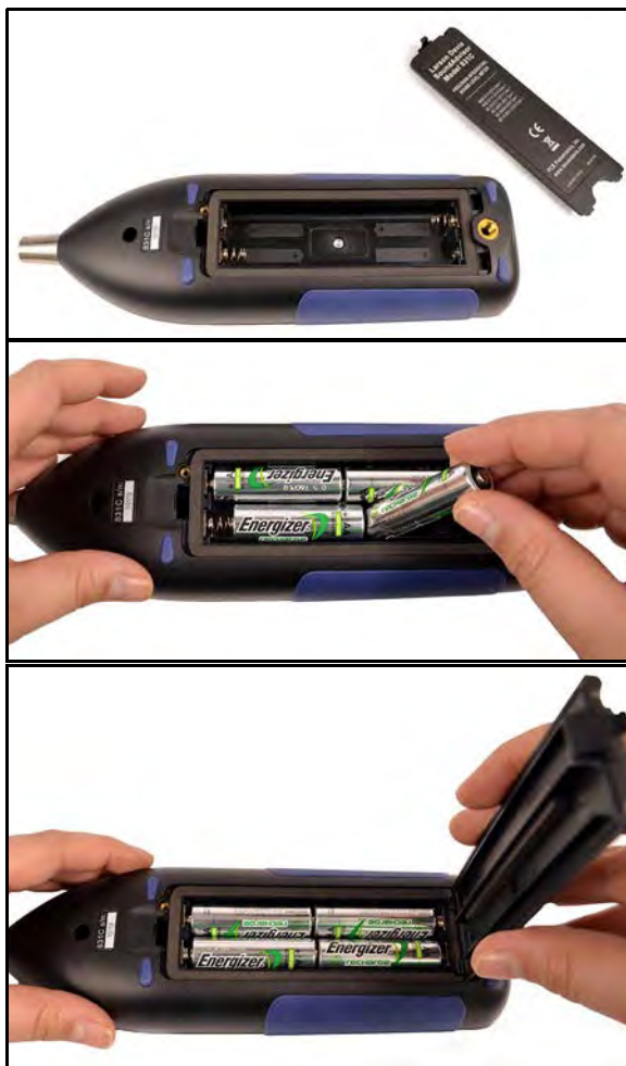
FIGURE 2-3 Installing batteries into the 831C.
