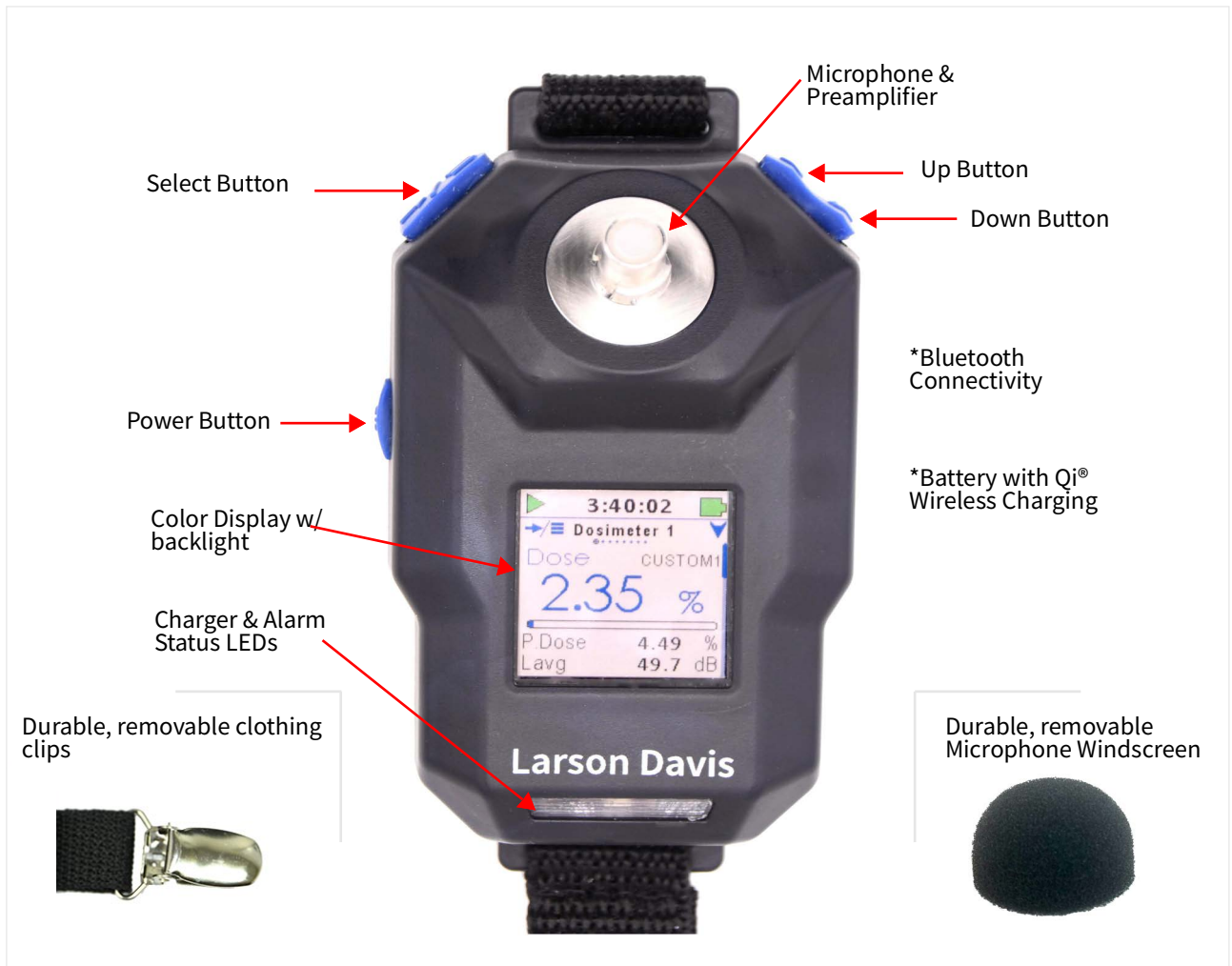
FIGURE 1-8 Components of the Spartan Model 730
