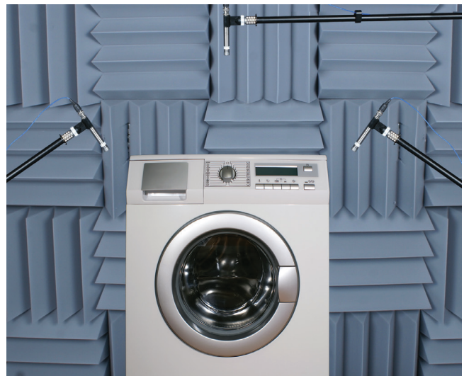
Sound Source Location for Noise Reduction
