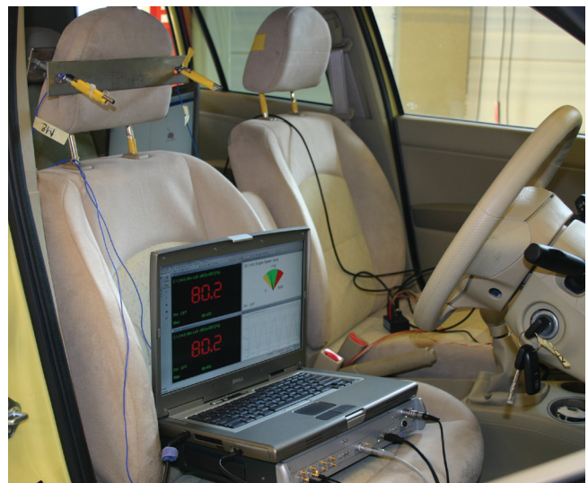
Cabin Noise Measurements for Rider Comfort
