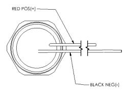
Figure 1 – wiring: standard connection
