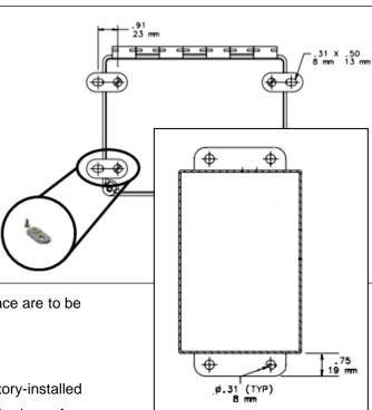
Painted steel and stainless steel boxes include two factory-installed mounting brackets on the top and bottom of the box. Hardware for
